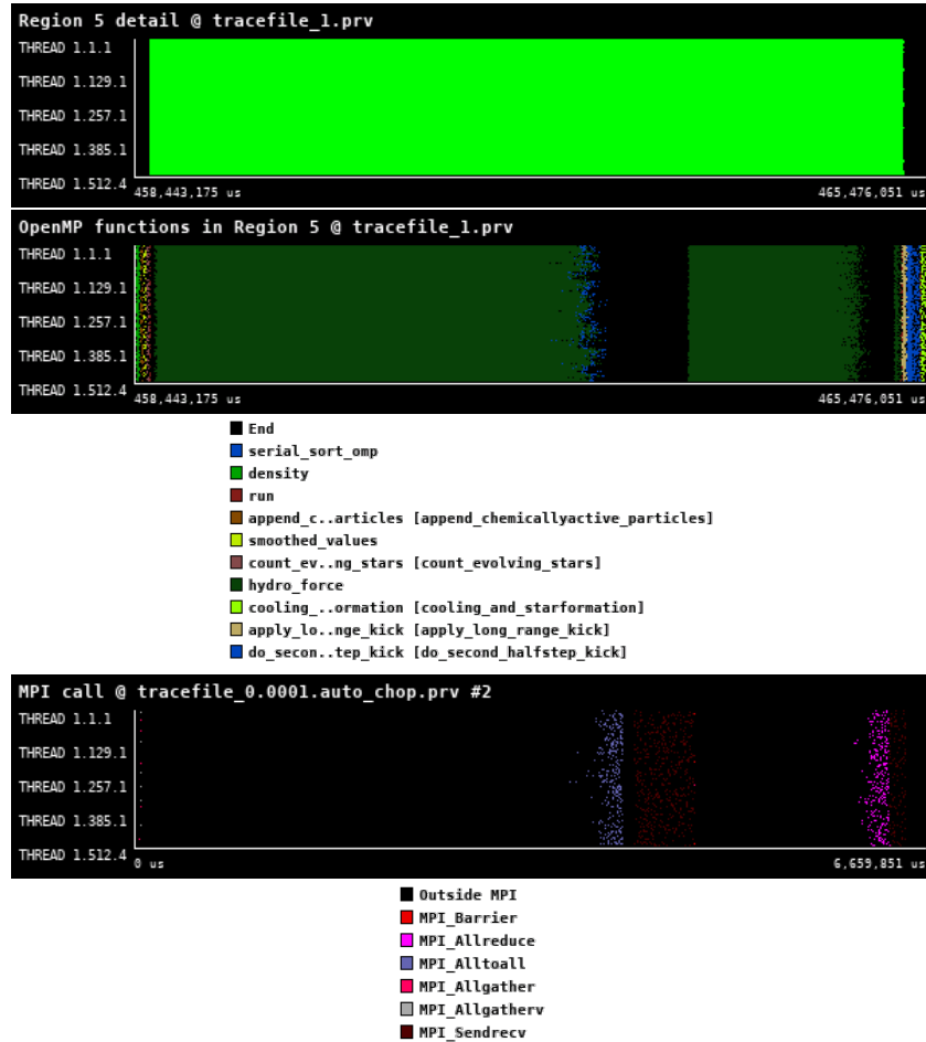
Figure 39: Zoomed traces for Region 5 of the Gadget from Paraver showing the structure of the region.
