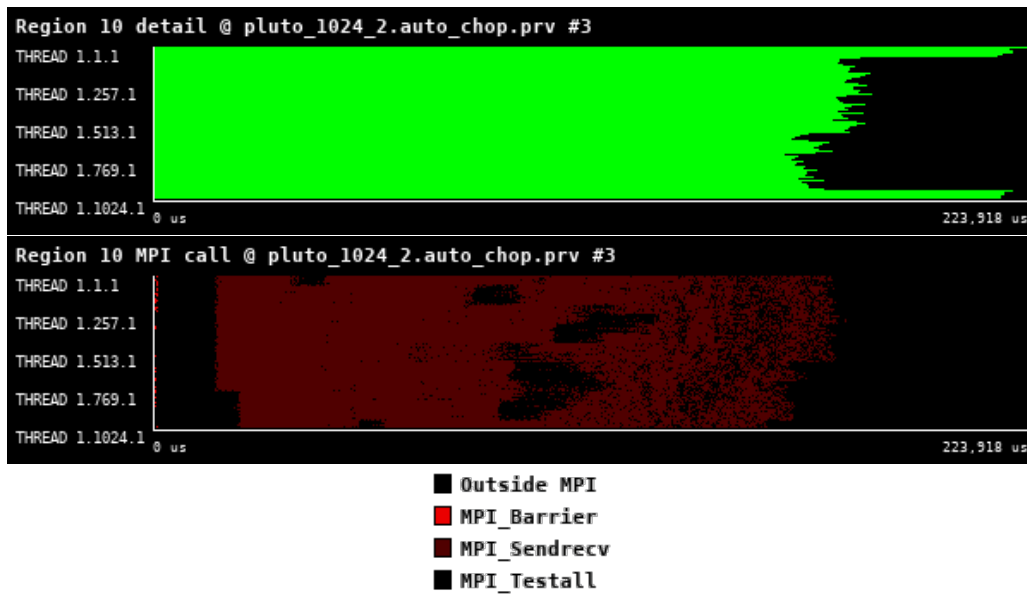
Figure 23: Zoomed traces for Region 10 of the PLUTO from Paraver showing the structure of the region.
