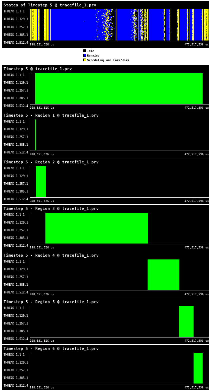
Figure 28: Traces for all regions in Gadget from Paraver showing the high-level structure of the code.
